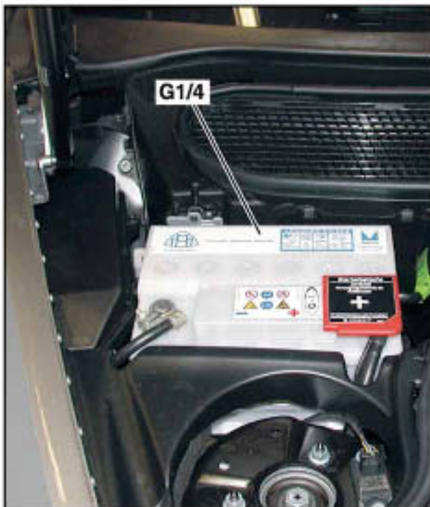
G1/4 Starter battery on right side of engine compartment
