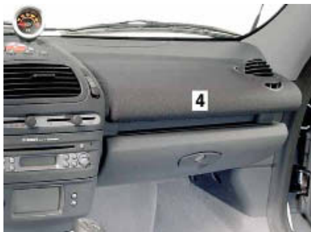
4 Front passenger airbag on smart roadster (model 452) and smart forfour (model 454)
